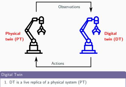
2. DT is connected to PT in near real-time via data streams
